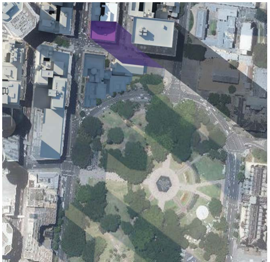
OVERSHADOWING GENERATED BY EXISTING BUILDING
